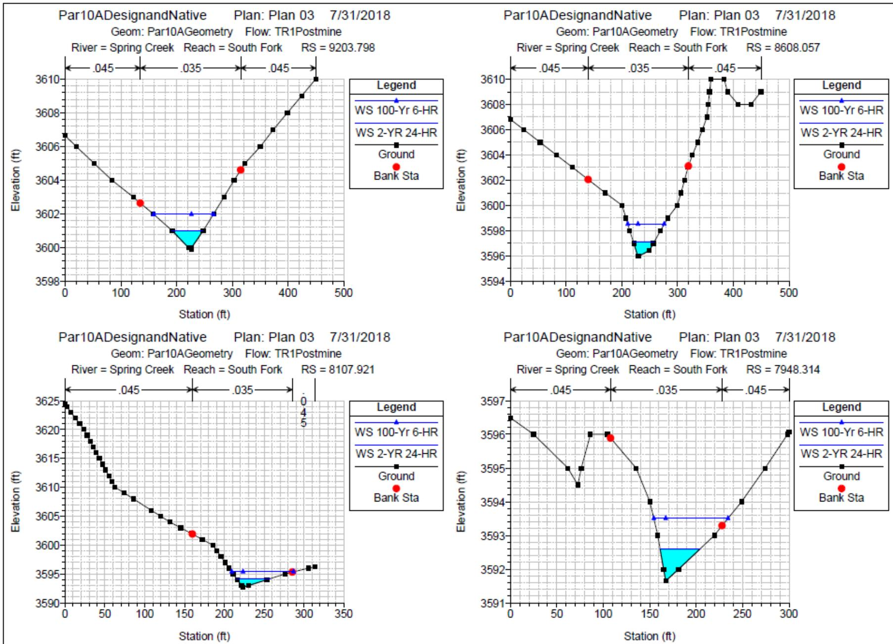
Figure 5. PAR 10A South Fork Spring Creek channel design segment HEC-RAS cross-sections
