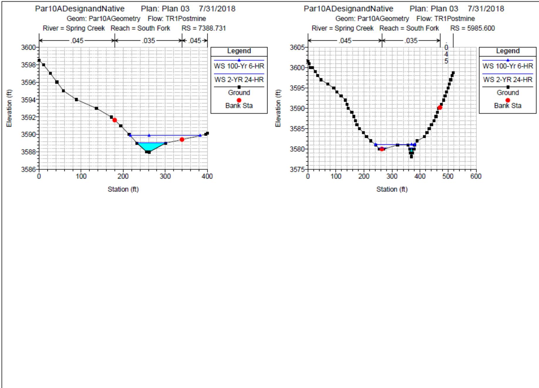
Figure 6. PAR 10A South Fork Spring Creek channel design segment HEC-RAS cross-sections
