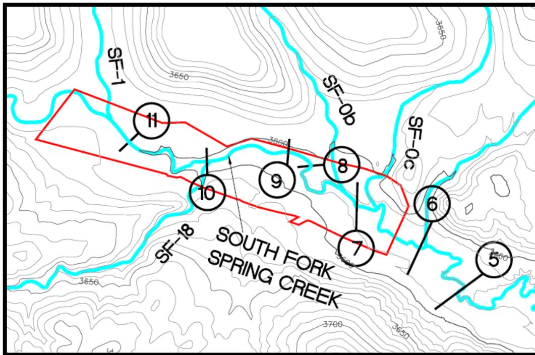
Figure 3. From Plate J-4, conceptual post-mining HEC-RAS cross-section locations with PAR 10A boundary in red.
