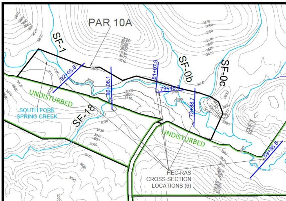
Figure 4. PAR 10A design topography with HEC-RAS cross-section locations in blue. Contour interval is five foot inside PAR 10A boundary and ten foot outside the PAR 10A boundary.
