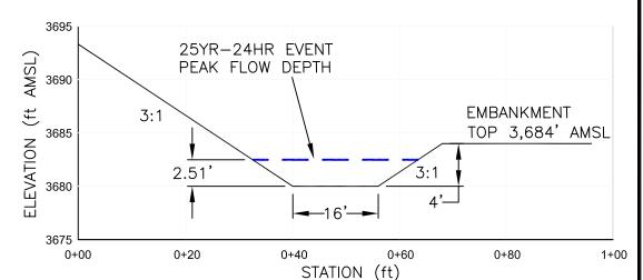
**TYPICAL SPILLWAY PROFILE** SCALE: H: 1"=40', V: 1"=10'
